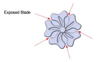
A tip from Carol at The Granary in Sunnyvale, CA: if you take the blade holder case apart and rotate the blade over one notch you get an additional 5 places on the blade to cut. You can do this twice, so you have a total of 15 places on the blade that you can use for maximum blade usage!
