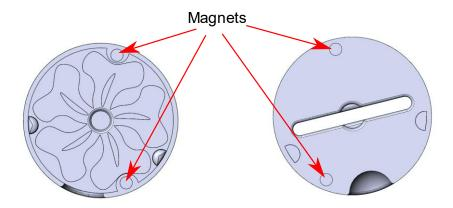
4. Also note that there are thumb holes in the top and bottom of the case. They make it easier to open the case, and they also make it easier to see how to align the case so the magnets and tabs snap into place.
