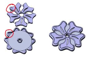
4. Next locate the **base of the bolt** (this piece doesn't have a screw hole in it).
