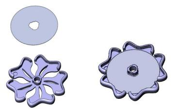
3. Next place the **blade cover** on top of the blade. Note that there is a small half circle cut out of one of the petals of the **blade holder bottom** and a small half circle cut out of the blade cover. Align the two halves of the circle and your cover will fit perfectly.
